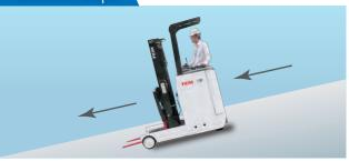
Maintains a constant safe speed (by suppressing acceleration on slope descent).
