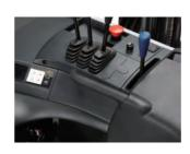
The steering wheel and the levers are oriented to ensure the comfortable posture during operation.
